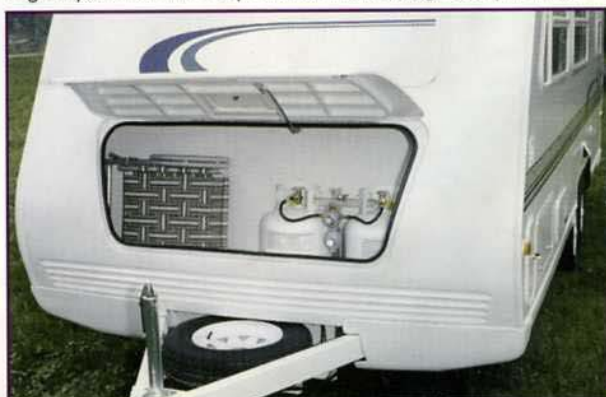
High Impact ABS Front Cap Creates Front Storage Compartment
